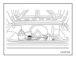
Include an ice scraper, a small brush or broom, a supply of windshield washer fluid, a rag, some winter outer clothing, a small shovel, a flashlight, a red cloth and a couple of reflective warning triangles. And, if you will be driving under severe conditions, include a small bag of sand, a piece of old carpet or a couple of burlap bags to help provide traction. Be sure you properly secure these items in your vehicle.
